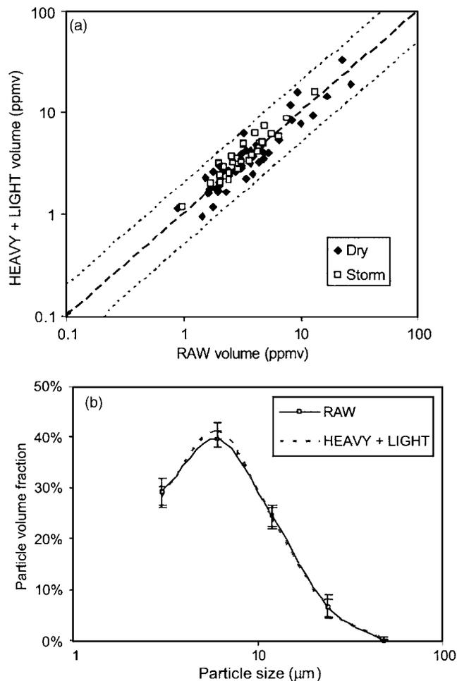
**Fig. 6.** Comparisons of particle suspension fractions: (a) total particle volume measurements from dry weather (diamonds) and storm (squares) samples plotted along with lines representing 1:1, 1:2, and 2:1 relationships ( $N=78$ ); (b) average particle size distributions for fractions from dry weather samples ( $N=48$ ): Raw (solid line) and Heavy + Light (dashed line). Error bars represent  $\pm 1$  standard error.
