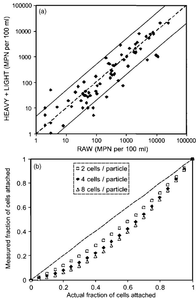
**Fig. 4.** Assessment of use of IDEXX for determining fractions attached to particles: (a) comparison of Raw concentration with sum of Heavy and Light plotted along with lines representing 1:1, 1:5, and 5:1 relationships; (b) calculated error due to multiple cells attached to individual particles in water sample. Dashed line represents 1:1 curve.
