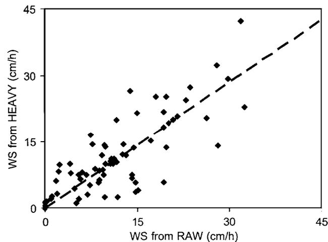
**Fig. 7.** Comparison of suspension settling velocities (WS) from Raw and Heavy samples. Linear regression (zero intercept with slope of  $0.94 \pm 0.04$ ,  $r^2 = 0.87$ ) plotted with measurements.
