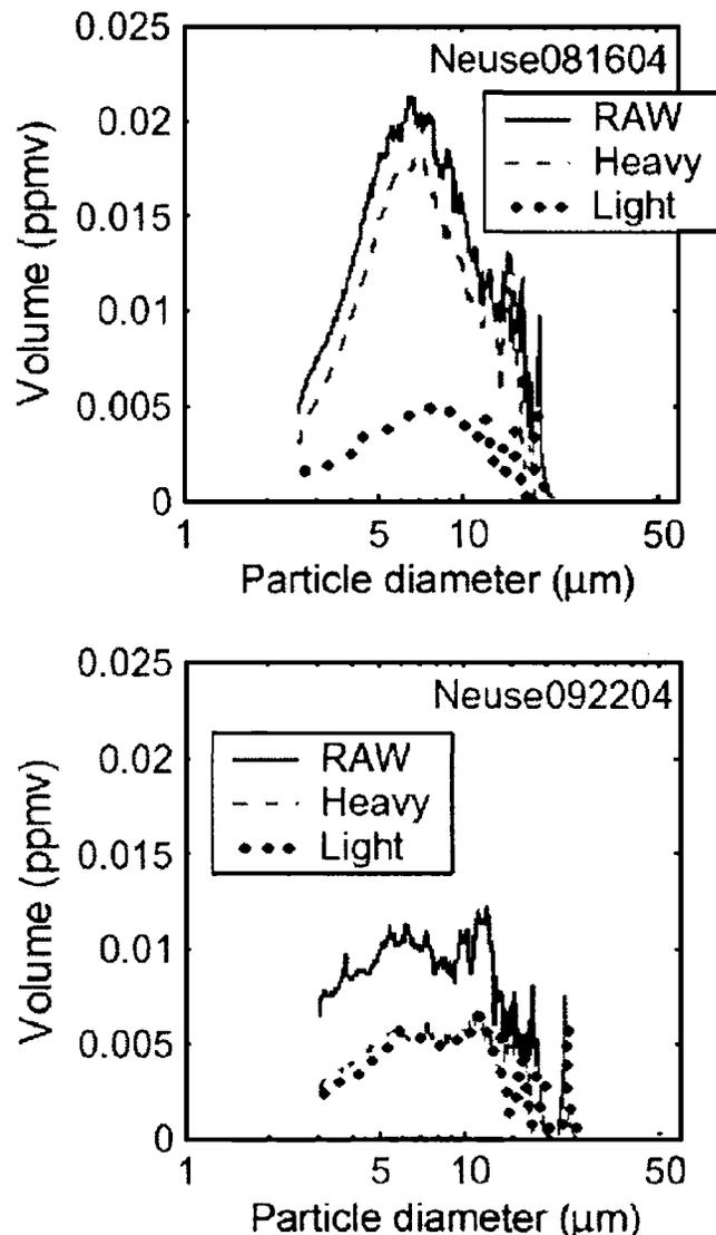
**Fig. 5.** Particle size distributions from surface water samples collected at Station 30. Top panel shows suspension from storm sample dominated by Heavy, likely runoff particles, and bottom panel shows mixed suspension of Heavy and Light particles from dry weather sample.
